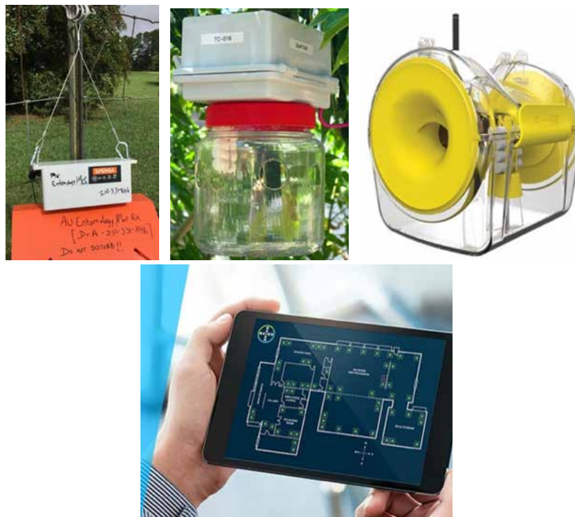
Figure 9 Examples of smart traps: left to right, DTN Smart Trap, Snap Trap, RapidAIM’s smart trap, Bayer’s RMS
